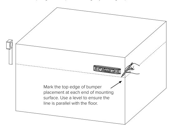
Measure case to determine base length. Allow an offset of 13/4" for end caps and 11/8" for corners.
