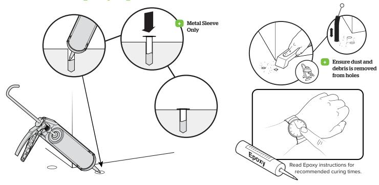
🕒 Remove plastic anchor and insert stainless steel sleeve into epoxy-filled holes until flange sits flush with the floor
