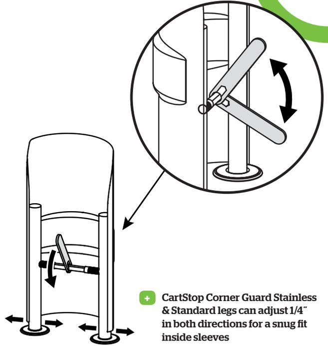
+ CartStop Corner Guard Stainless & Standard legs can adjust 1/4" in both directions for a snug fit inside sleeves
